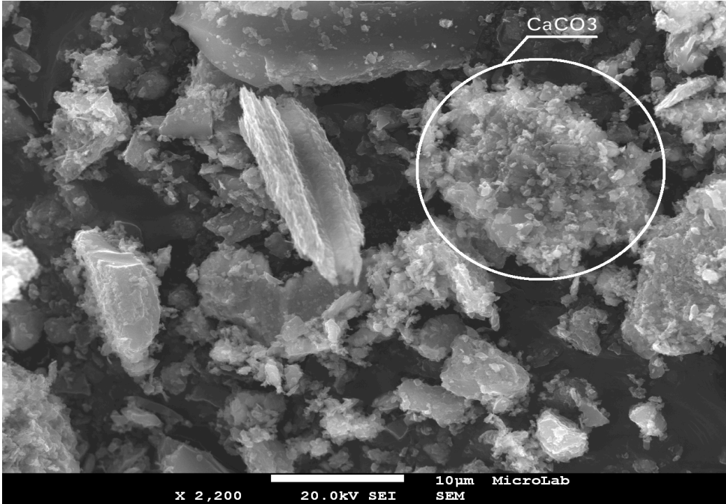
Figure 33. SEM picture of limestone (3% wt ) particles distribution on the coal char surface.
